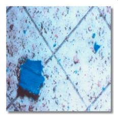
Sample #2 The second photo shown here is a sample of oil taken from a test unit with 10 micron filtration.
